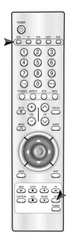
Press the appropriate button among the Component Selection buttons to activate another component (STB, TV, VCR, CATV, DVD). For example, if you want to program the remote control to operate your VCR, press the VCR button on the remote control.
